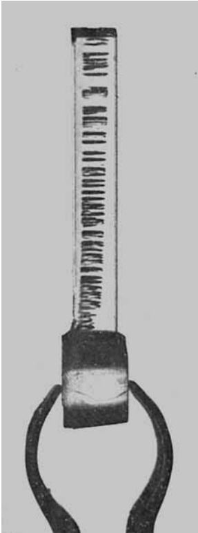
Fig. 4. Polystyrene test bar after rapid straining showing internal craze planes.
